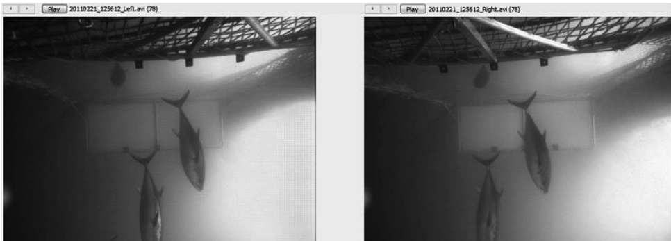
FIG. 1. Typical stereo-image pair captured during a transfer from the purse-seine net to the grow-out cage. The water surface is to the right of the images and the apparent vertical orientation of the fish is caused by the mounting of the stereo-video system on the side of the transfer gate.
