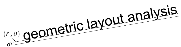
Figure 1. An illustration of Roman script text-line model proposed by Breuel. 12 The baseline is modeled as a straight line with parameters (r, \theta) , and the descender line is modeled as a line parallel to the baseline at a distance d below the baseline.
