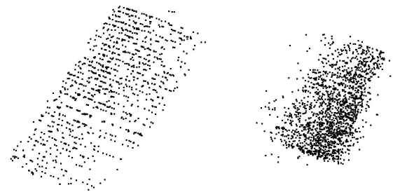
Figure 4. 3D reconstruction of book page with RANSAC. Left side shows the proposed method. Right side shows default matching.
