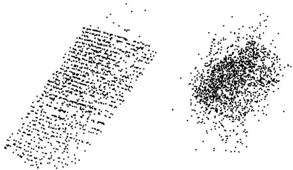
Figure 3. 3D reconstruction of book page without RANSAC. Left side shows the proposed method. Right side shows default matching.
