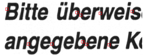
Fig. 4. Incorrect chosen windows due to an italic font. The windows are often selected from round or askew "edges".
