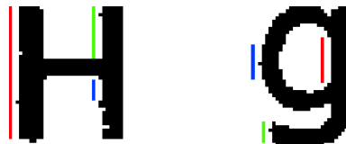
Fig. 2. Example of vertical edge detection. In both example characters the red edges are the longest and used for feature extraction.
