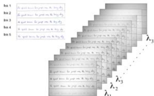
Fig. 3. A multispectral image stack written with five different blue inks and the corresponding RGB image.
